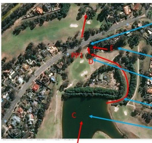
NOTE:- At Pinch Point 1 (PP1) debris from a dam collapse would create a dam at the drain under Heritage Way, this location there are no issues of water egress into residential properties as any damming effect at PP1 would simply overflow across Heritage Way.
