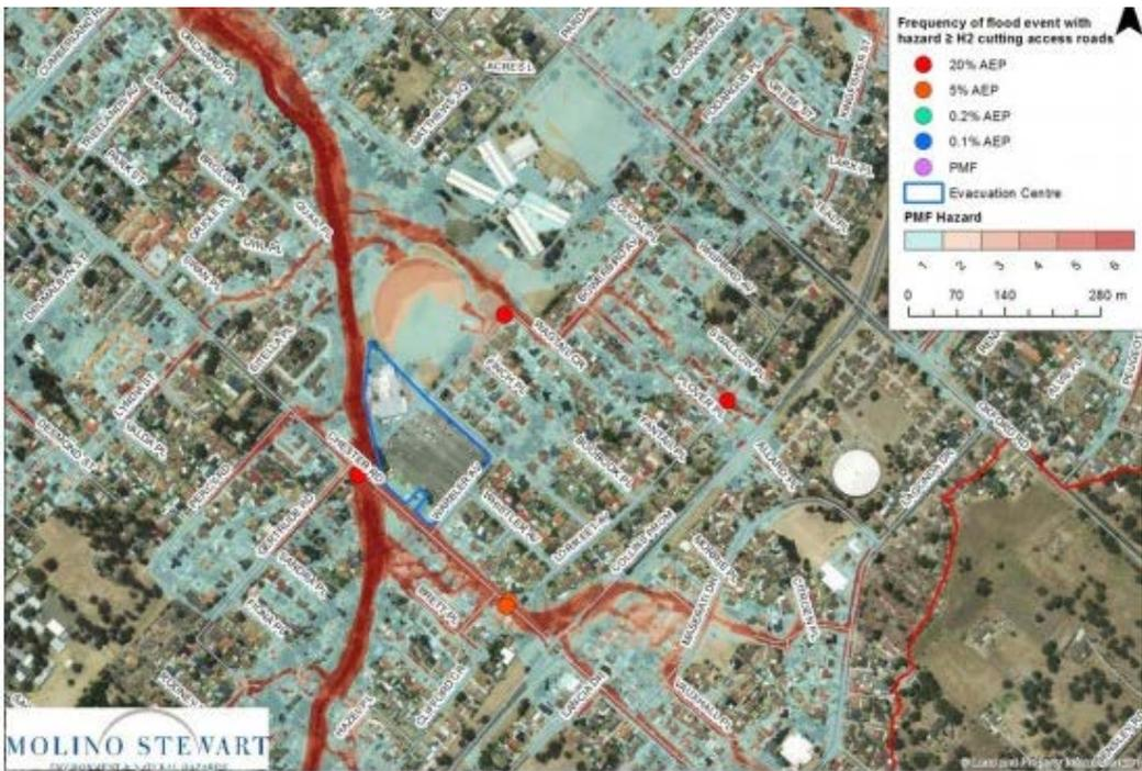
Figure 30. Flood risk to the proposed evacuation centre at Ingleburn RSL.
