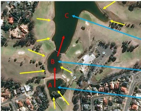
NOTE:- At this location there are no issues of water egress into residential areas with the collapse of a dam as Dam A runs downhill into Dam B.
