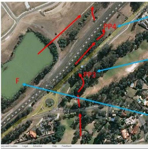
Water and debris passing PP4 will flow into an open lined drain that will eventually reach Bow Bowling Creek.
