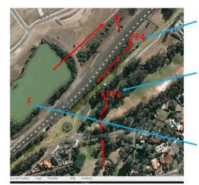
Water and debris passing PP4 will flow into an open lined drain that will eventually reach Bow Bowing Creek.
