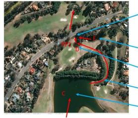
NOTE:- At Pinch Point 1 (PP1) debris from a dam collapse would create a dam at the drain under Heritage Way, this location there are no issues of water egress into residential properties as any damming effect at PP1 would simply overflow across Heritage Way.
