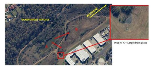
If Dam A were to collapse water would flow into Retention Basin at "B". Water in the retention base would flow towards a large drain grate shown at Insert A. It is considered that during a storm event the drain at Insert B could become blocked.
